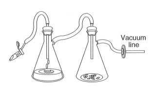
An aspirator used for potentially infectious material must be equipped with a hydrophobic filter between the flasks and the vacuum supply. This prevents the uptake of material into the vacuum system. If the vacuum suddenly is reduced, it is usually because the filter has become wetted and must be replaced. Be sure you know where the replacements are.
